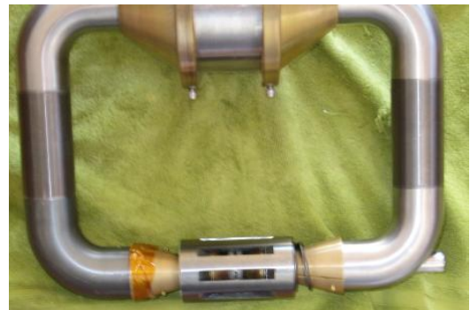
Figure 11. Magnetic core with lithium sapphire cell installed, but without superconducting coil .
