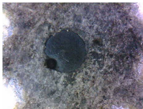
Fig 19. B4C and Lithium after cavitation
