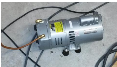
Figure 13. Carbon vane vacuum pump.
